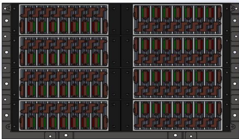
Fig 69:CAD Rendering of cells in the battery box with transparent Lexan sheet on top.
