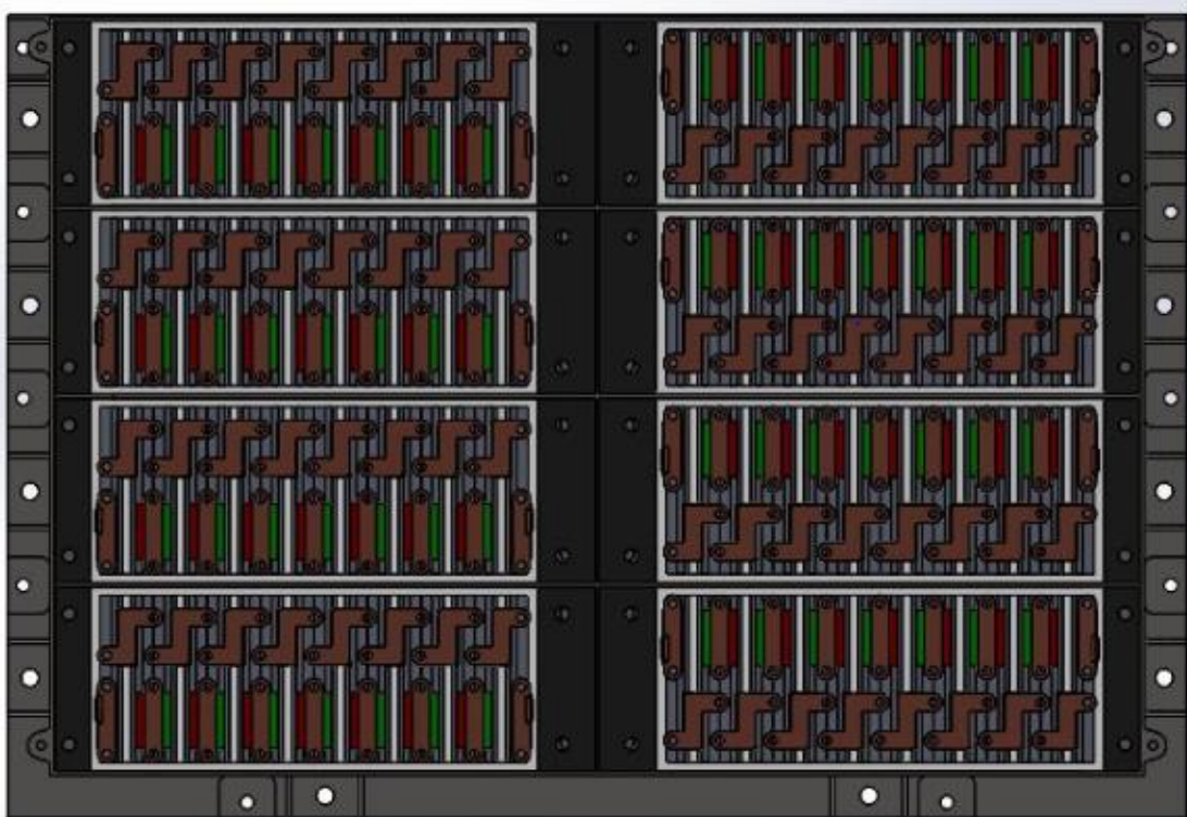
Fig 69:CAD Rendering of cells in the battery box with transparent Lexan sheet on top
